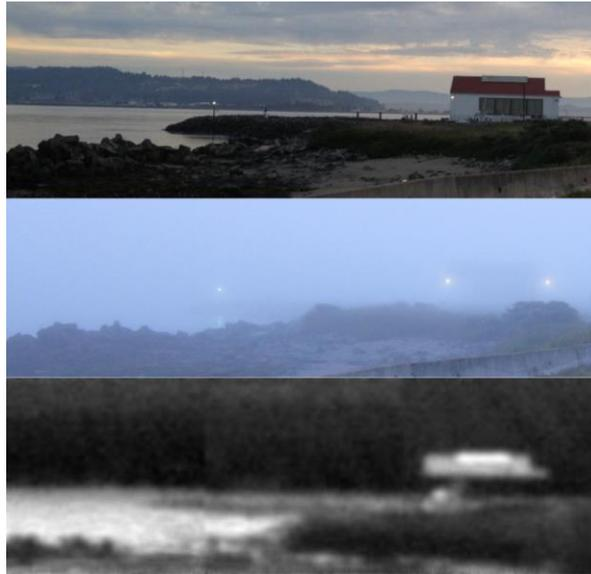
Figure 1.2: Visible image of a building on a clear day (top) and the same building on a foggy day (middle) and a millimeter wave image of the building in the same fog (bottom).
