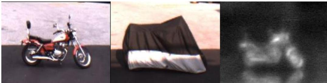
Figure 1.3: Imager of (left) a motorcycle in the visible light spectrum and (middle) a motorcycle with a cover in the visible light spectrum and (right) a millimeter wave image of motorcycle with a cover.
