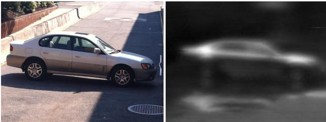
Figure 7.1: (a) Visible image of a car, (b) 77 GHz image of the same car.
