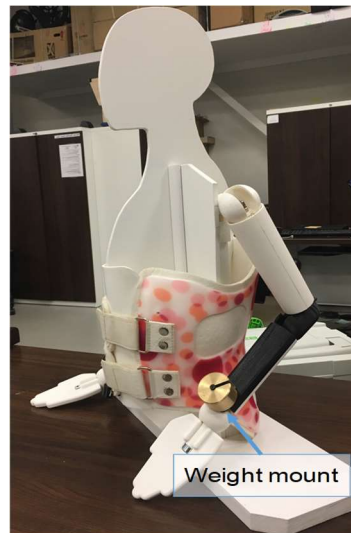
Figure 5.3 The designed and 3D printed upper extremity phantom model.
