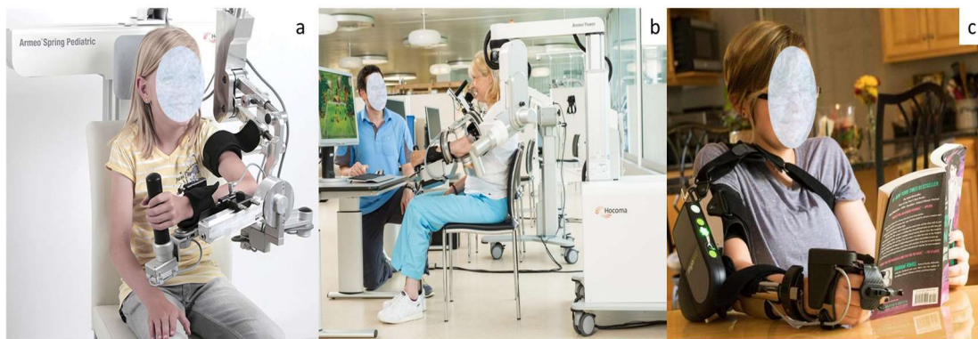
Figure 5.1 Example of commercially available exoskeletons (a) Armeo Spring.(b) Armeo Power.(c) Myomo. The Armeo devices, although versatile, are bulky, expensive and complex.
