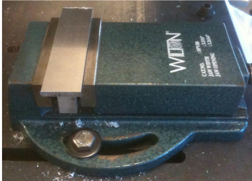
Figure 3.4. Image of the vise used during UC holding a substrate.
