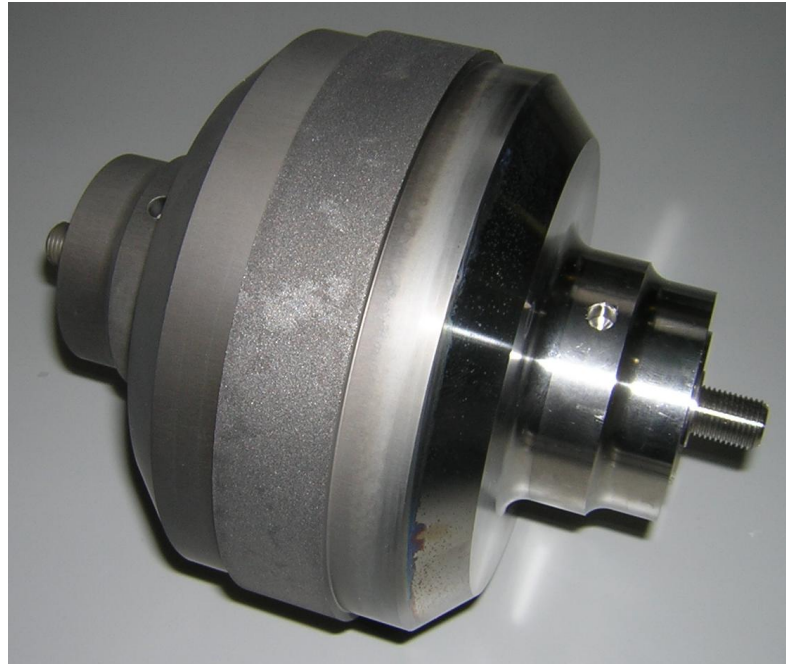
Figure 3.2. Image of the EDM textured sonotrode.
