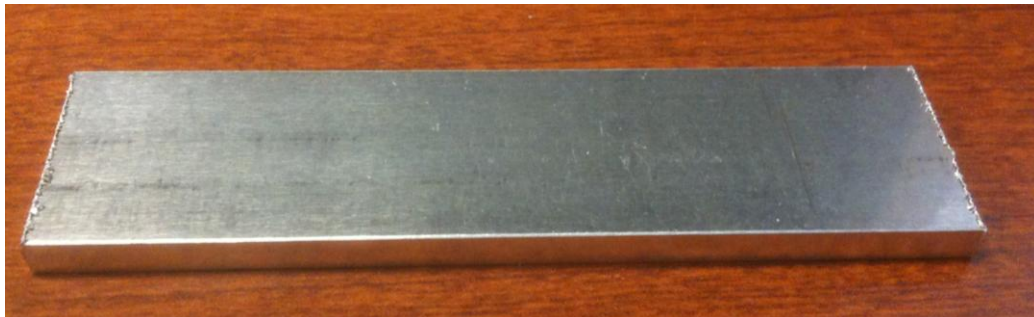
Figure 3.10. Image of the Al 3003-H14 substrates used during UC (26.5mm x 4.76mm).
