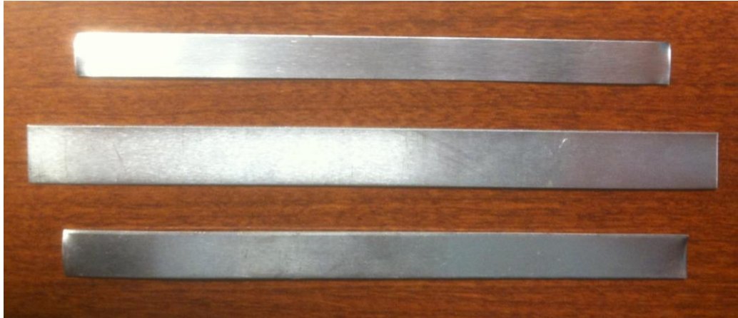
Figure 3.9. Image of the three Al 1100-0 foil geometries used during UC. The dimensions are 9.5mm x 0.52mm (top), 13mm x 0.52mm (middle), and 9.5mm x 1.04mm (bottom).
