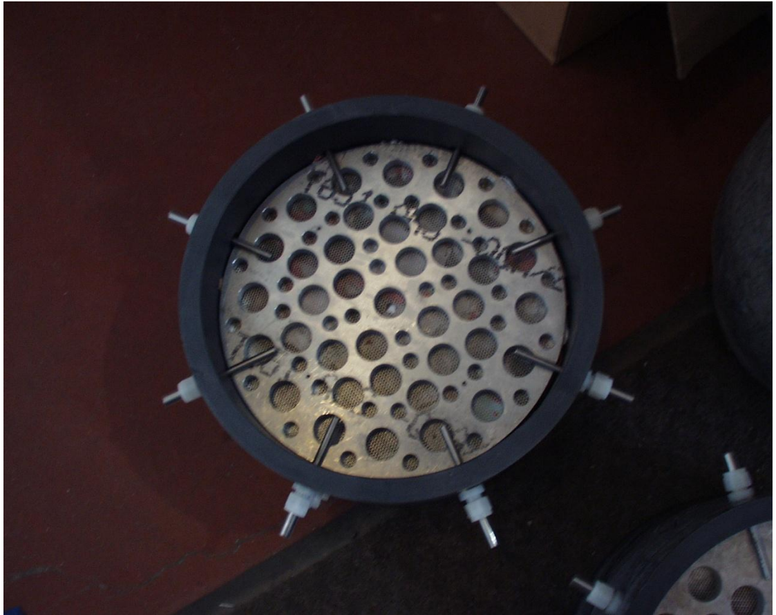
Figure A.5 Completely compressed waste column with top plate and support rods.
