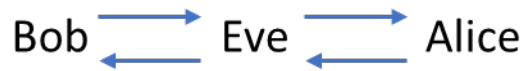
Figure 3 Bob and Alice communicate over a monitored network controlled by Eve. Bob and Alice send data back and forth, while all data must go through Eve. Usually, Bob is trying to send some message to Alice. Alice is usually trying to tell Bob she received the message.
