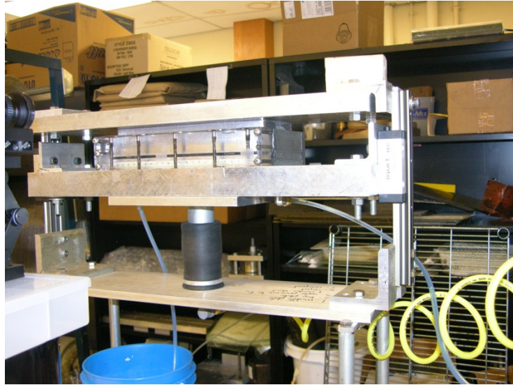
Figure 7-12 Experimental setup used to compress the partially filled preform under constant applied force
