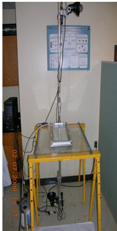
Figure 3-9 Experimental setup to measure through thickness permeability by recording the advancement of the flow front at the top and the bottom surface of the mold.
