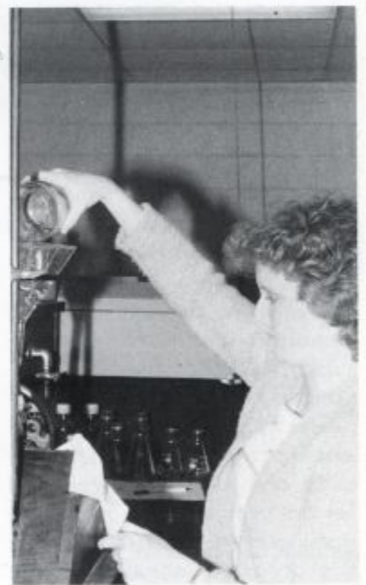
In a textile performance lab, Maryan Connery pours water onto a piece of fabric to test its resistance.
