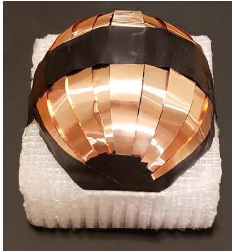
Figure 5.13: View of the copper tape placed over the spherical end cap of the reflector.
