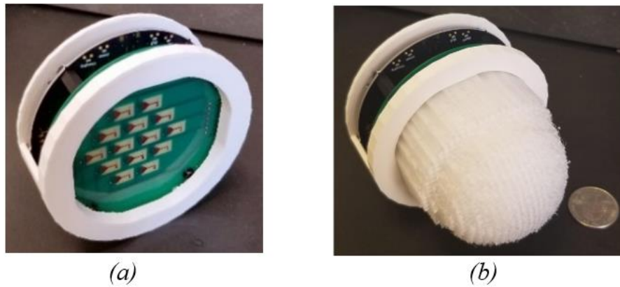
Figure 5.24: Overview of power detecting system. (a) Close up of antenna matrix. (b) Microcontroller/BT, battery, PCB antennas, and Luneburg lens enclosure.
