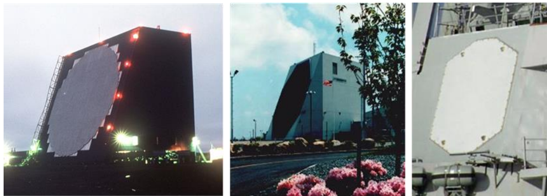
Figure 1.1: Images of the (left to right) Cobra Dane [3], PAVE PAWS [4], and SPY-1 [5] radar systems
