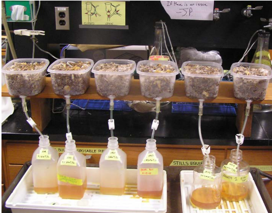
Figure 2. Biocell reactor setup. Reactor chambers R1-R6 (left to right) are filled with P. ostreatus inoculated mushroom compost. Influent is being supplied via three peristaltic pumps from the large Erlenmeyer flasks behind the reactors. Effluent is being collected in the bottles towards the bottom of the picture.
