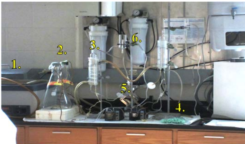
Figure 1. Packed-bed bioreactor setup. A heated water bath (1) warms the reactor chamber (3). This chamber is then filled with inoculated media, in this case foam cubes (4) and the influent is pumped into it through the reservoir tanks (2). The solution is simultaneously aerated by small aquarium pumps fitted with .2 \mu\text{m} filters. Two peristaltic (5) pumps provide the influent and effluent flow. The column on the far right (6) allows for recycle flow.
