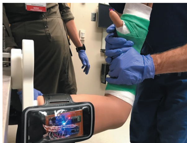
Figure 5. Distal radius fracture model arm and exterior processing and computing hardware in use during a trial reduction and casting experiment.
