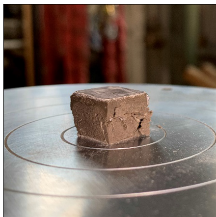
Fig. 7. Post-compression images of BP-1 binders showing differences in failure mechanisms, representative of all binders studied. Left: cube cured under ambient conditions, shows buckling in the center of the cube and compression. Right: cube exposed to high temperature, shows vertical cracking and shear failure.
