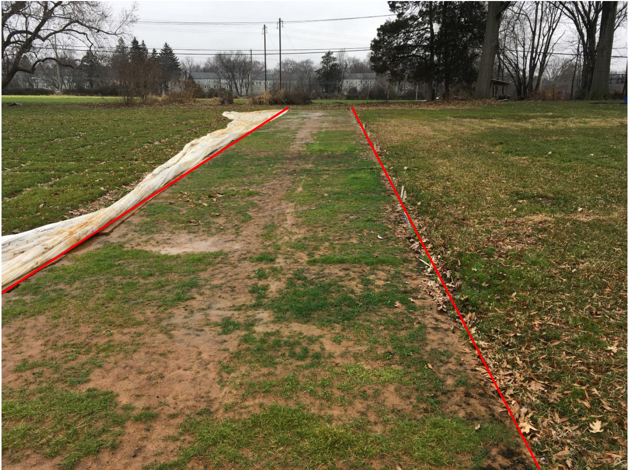
Figure 14 Sod over plastic 3 months after sowing. The sod is between the red lines.
