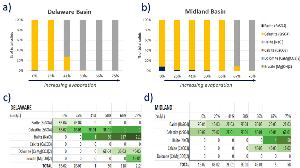
PHREEQC predictions of relative volumes of each salt crystallized as percent evaporation increases for the a) Delaware and b) Midland produced waters. Individual volumes (cm 3 /L) of each salt are also reported for the c) Delaware and d) Midland basin, with darker green being higher volumes.
