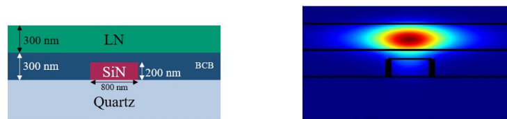
Figure 5.7: Optical simulation of waveguide, at 1064 nm, with 300 nm thick layer of BCB.
