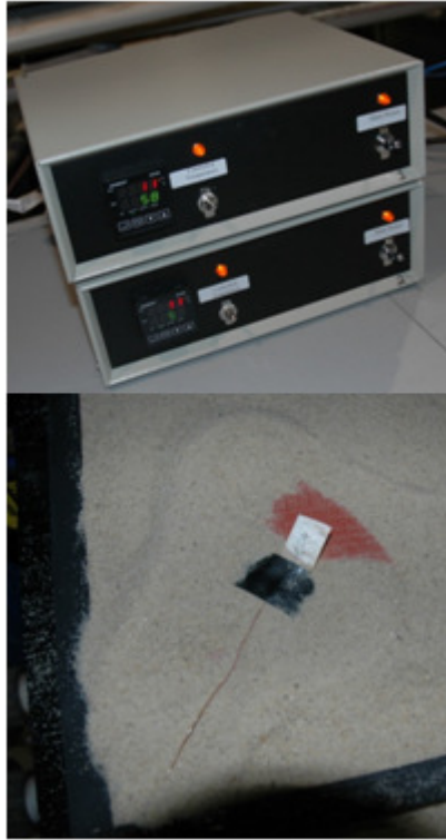
Figure 3.8: Omega Temperature Controllers (top) and Thermocouple (bottom)
