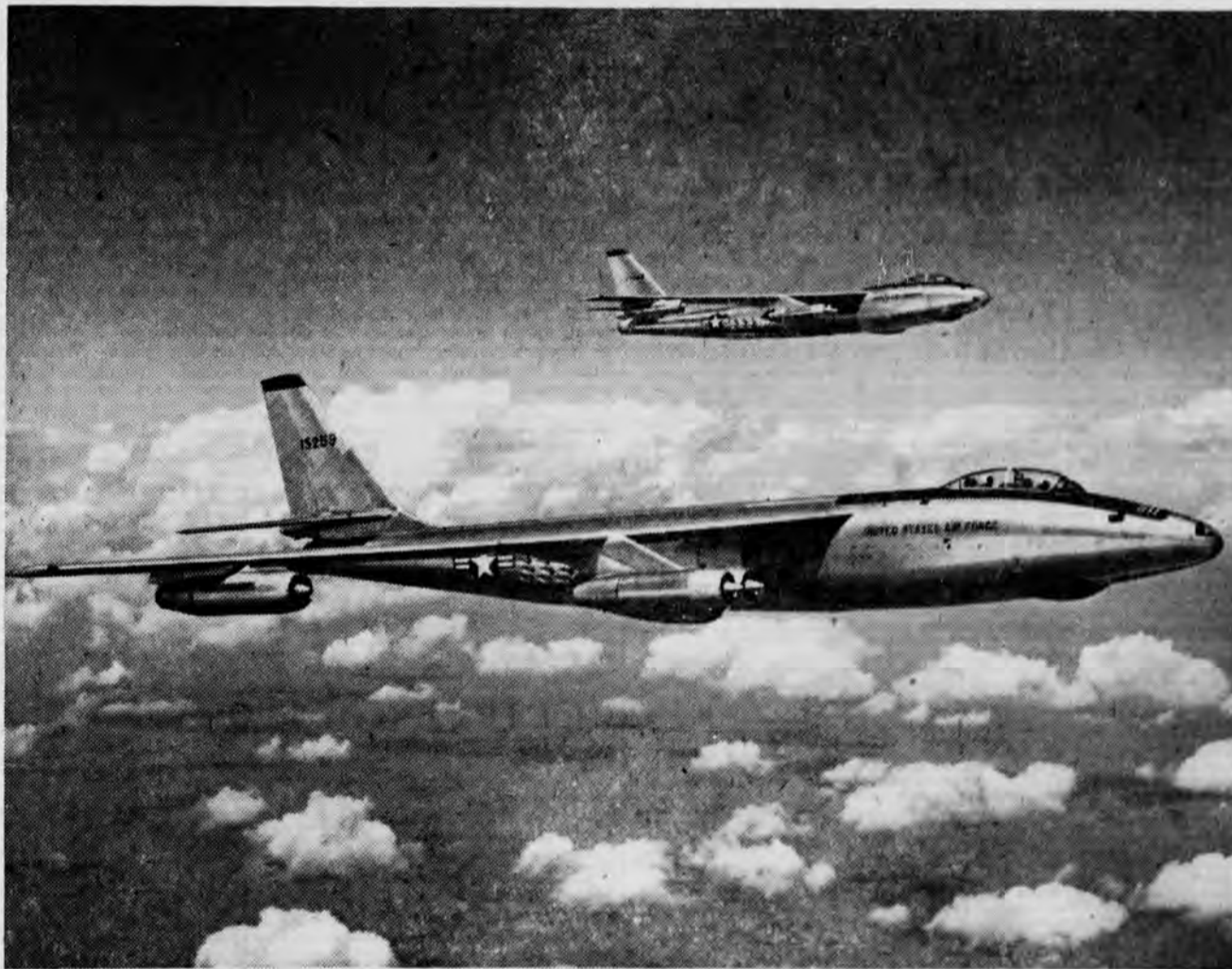
Foreground: Boeing RB-47E, world's fastest day-or-night long-range reconnaissance plane. Background: Standard B-47E six-jet bomber.
