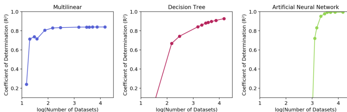
Figure 5.8: Number of datasets needed for each of a) multilinear regression, b) decision tree, and c) neural networks to generate models of a given accuracy
