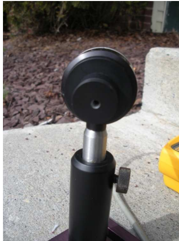
Figure 1.18 Photo detector with ¼” shield to block outside light
