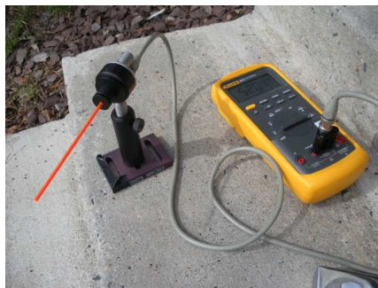
Figure 1.20 Overall setup, photo detector, fiber, and multi-meter.
