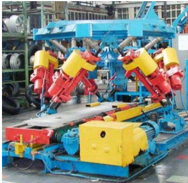
Fig. 1.2 Upgraded Gough Platform Tire Testing Machine used today
