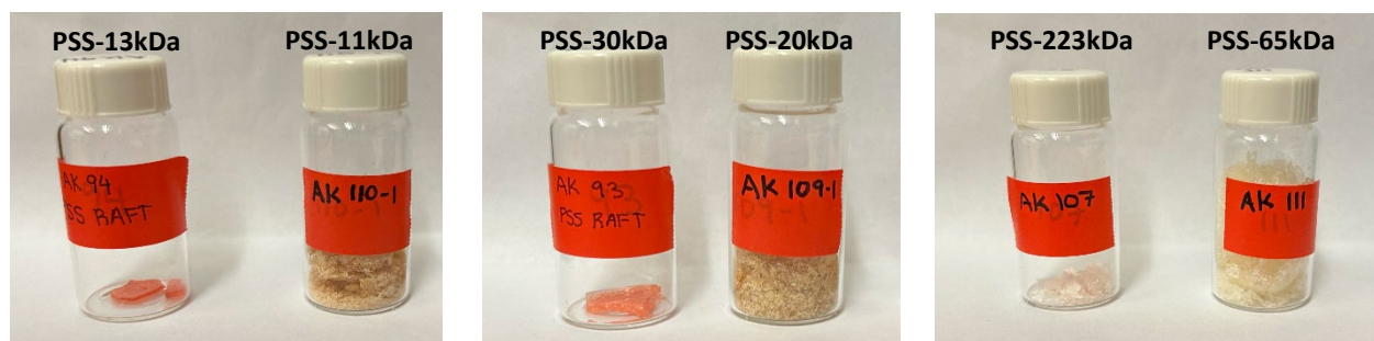
Figure S1. Color changes were observed after removal of the RAFT chain end group. The left vial of each pair is the original PSS synthesized with the end group still attached (PSS-13kDa, PSS-30kDa and PSS-223kDa). And the right vial of each pair is the corresponding final PSS sample, obtained after the cleavage reaction, with the end group removed (PSS-11kDa, PSS-20kDa and PSS-65kDa).
