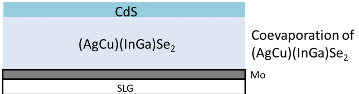
Figure 2.12 Deposition of absorber layer (ACIGS) by using coevaporation and buffer layer (CdS) by chemical bath deposition (CBD). This forms the p-n heterojunction.
