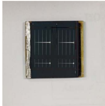
Figure 2.11 ACIGS piece with four cells. Cell areas are 1.00 or 0.4 cm 2 . The shiny white metal region on the left is an Indium solder used to connect the front metallic grid to Mo back contact of the cell.
