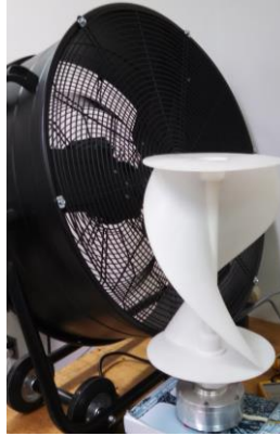
Figure 5.8 Image of the 24-inch blower fan and WT placement used to imitate the high level of wind speed (6 m/s).
