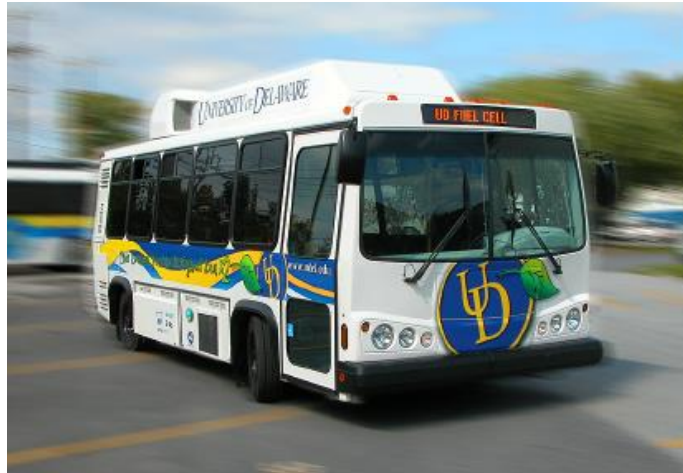
Figure 3.2 The University of Delaware’s 22-foot, 22-seat transit bus manufactured by EBus, Inc. of Downey, CA, and equipped with a fuel cell/battery series-hybrid powertrain.
