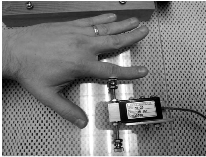
Figure 4.1: Custom force measuring device for index finger abduction.
