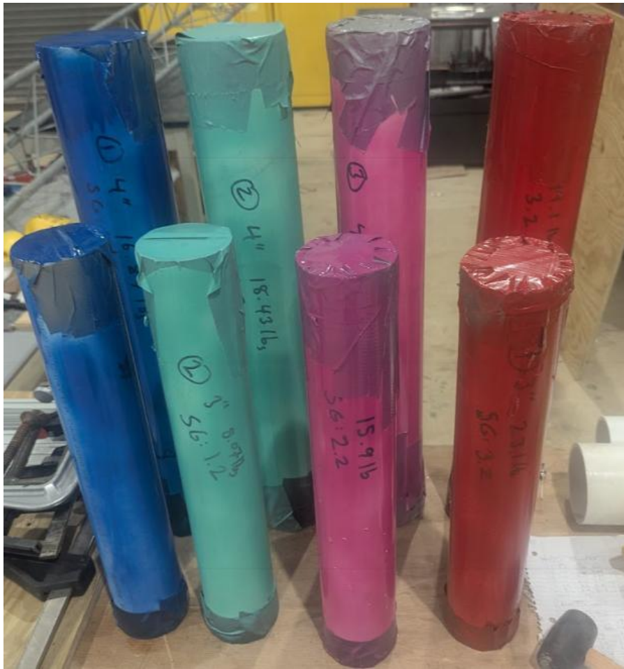
Figure 09. Finished targets prior to use in the experiment. Colors indicate SG (Blue = 1.1, Green = 1.2, Orange (unpictured) = 1.7, Pink = 2.2, Red = 3.2).
