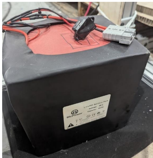
Figure 15. The BTR LiFeP04 Batteries (48, 60 Ah).
