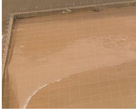
Figure 18. 10 cm x 10cm Grid System used for positioning targets.
