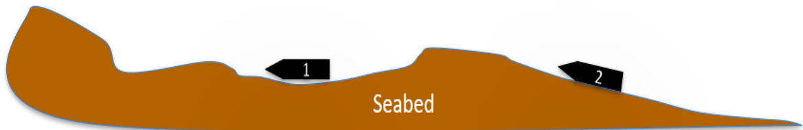
Figure 03. How local morphodynamics can effect munition stability. Munition 1 has much more local stability than Munition 2.
