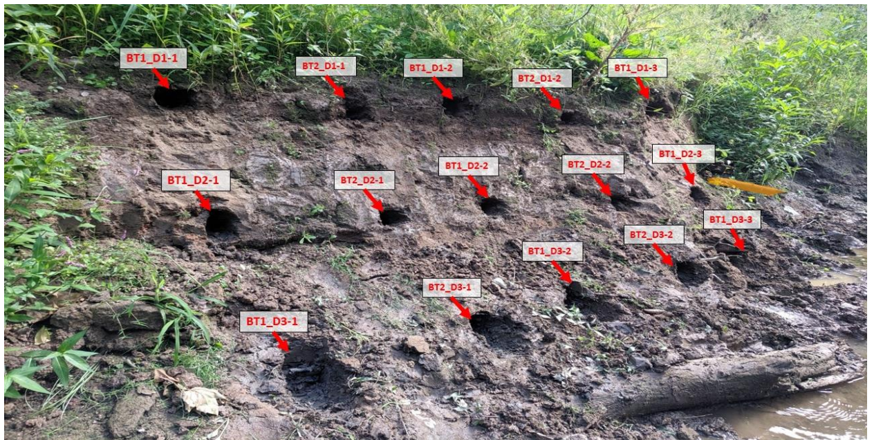
Figure 3.6: The relative locations of the Krady milldam terrace depth samples. Sample Identification can be understood as follows (BT1_D2-3 / Bridge terrace sample set 1, depth 2, subsample 3). BT2_D(1,2&3)3 not visible in the above image due to the angle of the photo.
