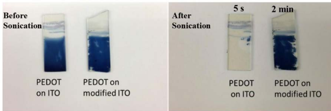
Figure 3.8 Optical images of PEDOT films on ITO and modified ITO before and after ultrasonication adhesion test. PEDOT on ITO was tested for 5 s and PEDOT on modified ITO was tested for 2 min (Wei et al. 2015).
