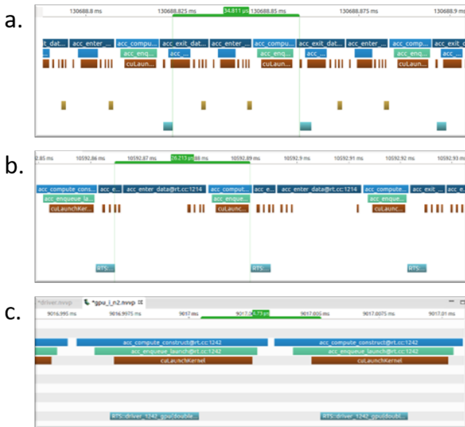
Figure 2.8: Nvprof profiler highlights the process of reducing kernel launch overhead in the RTS integrate() kernel. (a) Overhead between 2 launches, (b) Reduced overhead between kernels launches, and (c) Further reduced overhead
