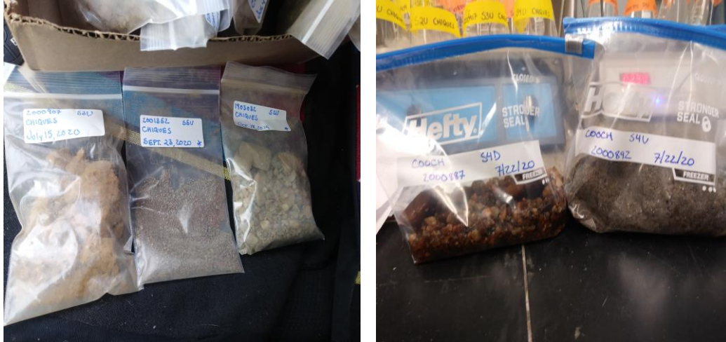
Figure 3.8: Images comparing streambed sediment from Chiques Creek (left) and Christina River (right) collected from various distances from dam and seasons. Note variation in sediment size and type.
