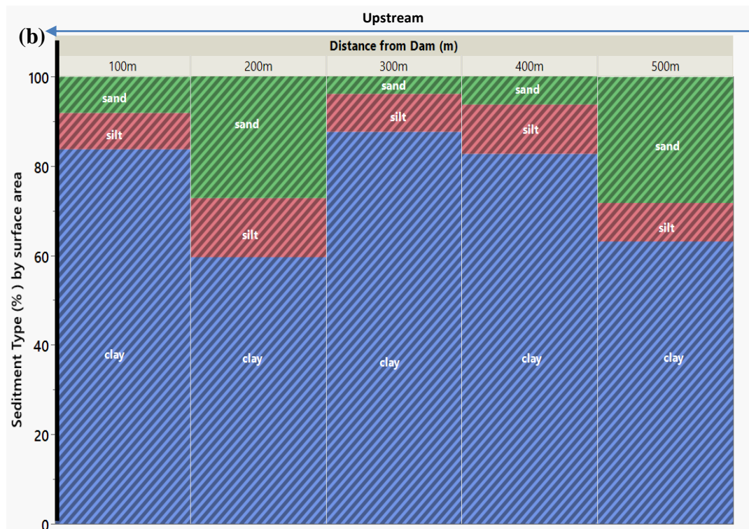
Figure 4.15. Percent sediment particle size by surface area and by distance from dam for Christina (a) and Chiques (b). Dam represented by black line. No sampling was done for Chiques downstream.
