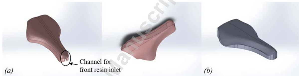
Figure 7. (a) Top (left) and bottom (right) views of the final elastomeric mask shape and (b) corresponding bottom mold shape.
