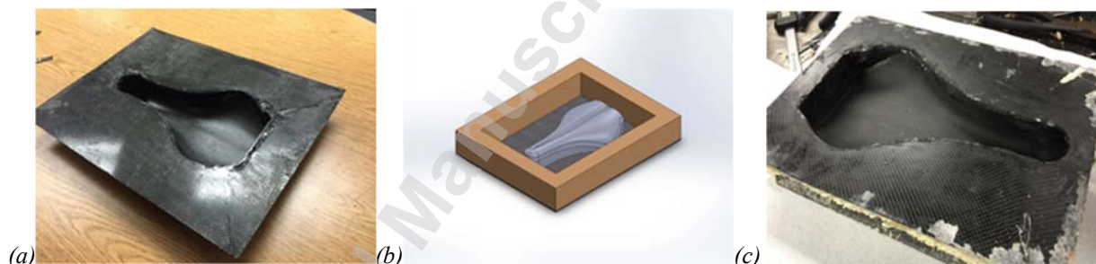
Figure 12. (a) bottom laminate skin, (b) pouring mold for mix-and-pour foam core, and (c) final top mold construction.
