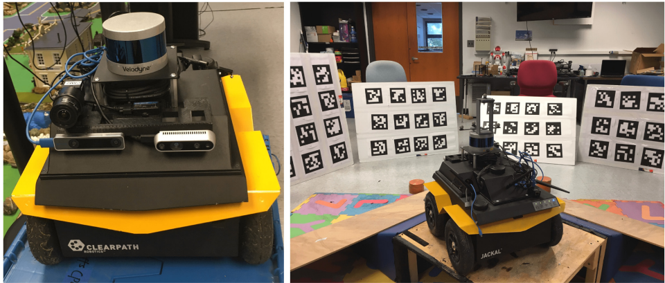
Fig. 5. Sensor setup for Jackal containing Velodyne VLP-16 LiDAR, Microstrain IMU GX5-25, Realsense T265 cameras, and FLIR Blackfly camera. Jackal itself contains a wheel encoder.
