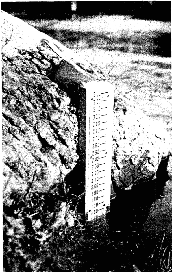
Figure 21.—Vertical staff gage.
