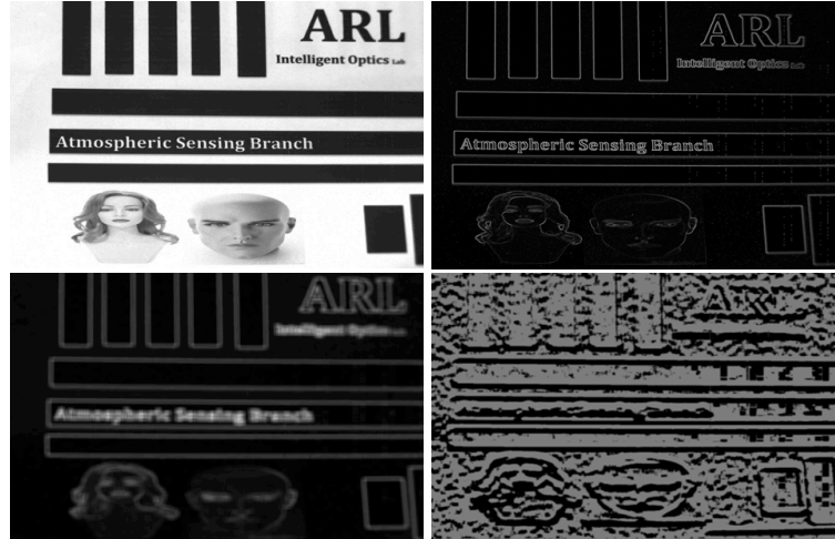
Figure 3.2: 1 st Generation Results. Top left is original image. Top right is image after Sobel Edge Detection. Bottom left is Image Quality Map. Bottom right is Keep Map.
