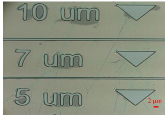
Figure 5.8: Optical Image of Agarose etched waveguides on sputtered Er-TeO 2 using HCl + HF+ IPA solution.
