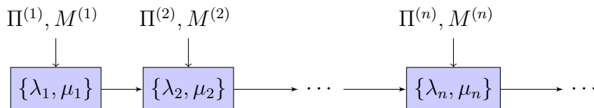
Figure 2.9: Flow chart of the algorithm presented in this paper. \Pi^{(n)} is the probability of left exit and M^{(n)} is the mean of the extinction times, all conditioned on that the particles remain in the domain of \{1, \dots, n\} before exiting. At each site, a pair of birth and death rate at that site is recovered.
