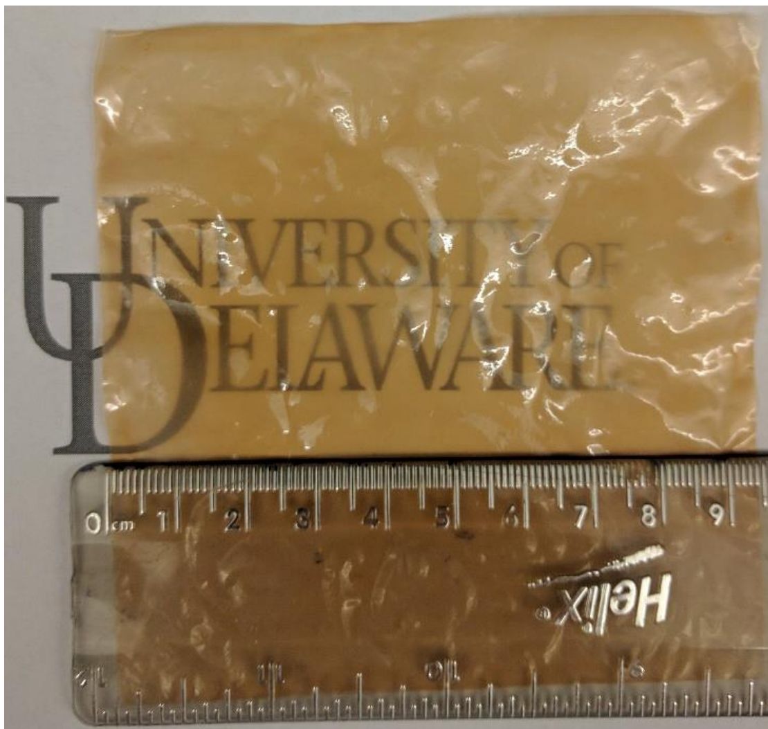
Figure 3.10: Prepared TTMPP-PBI-3/PTFE reinforced membrane. ePTFE was used as reinforcement support.
