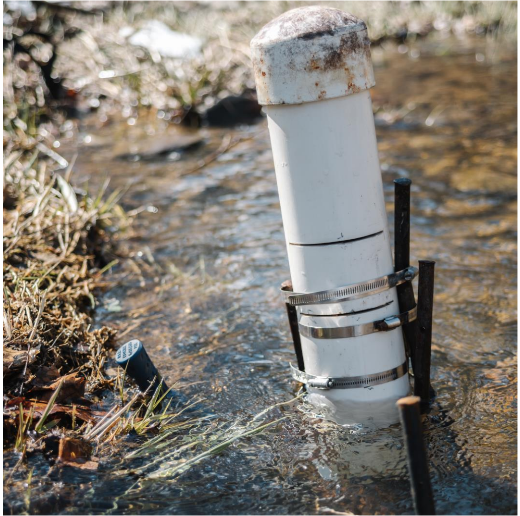
Figure A4: Passive sampler used to collect storm sediment samples at the Big Elk Creek, downstream site.
