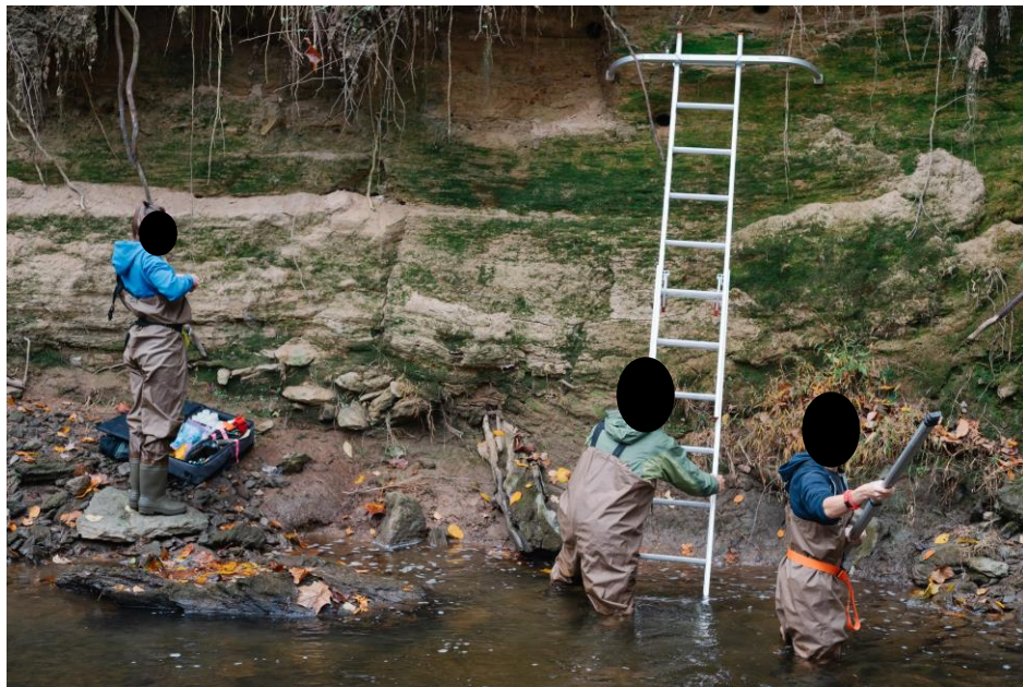
Figure A6: Sediment sampling at a legacy sediment impacted-stream bank within the Big Elk Creek.
