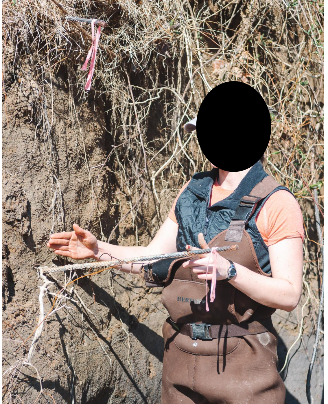
Figure A11: A lab member showing how much stream bank erosion was recorded by an erosion pin at the Big Elk Creek downstream site between the date of installation (8/3/2017) and the date of the photo (4/3/2019).
