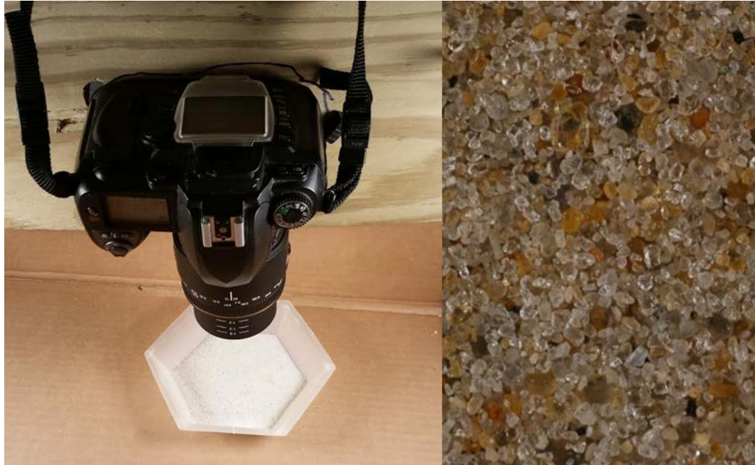
Figure 3.8 a) the stand of the camera, b) a picture of a typical sediment sample
