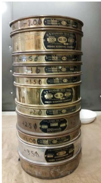
Figure 3.7 Stack of sieves that was used to obtain sediment grain size
