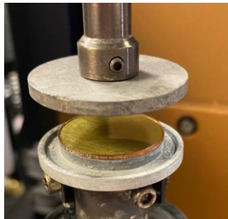
Figure A2. Polymer rheology setup with 25 mm diameter, 1 mm PEI disk loaded between two parallel plates.
