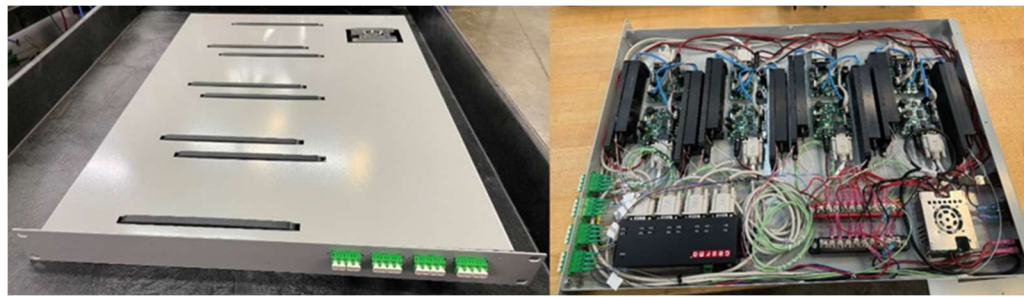
Figure 4.5. Left: A true time delay (TTD) box with lid on. Right: inside view of the enclosure.
