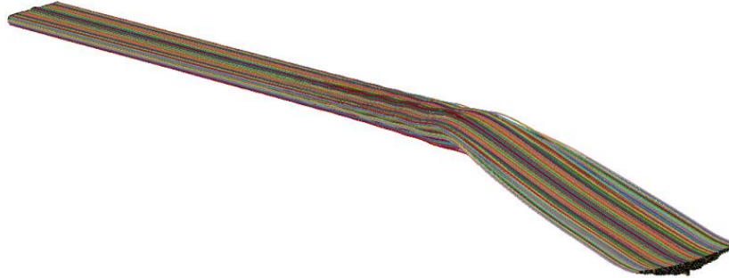
(g) Fiber-fiber interactions – spreading and flattening of fibers within a yarn 7
