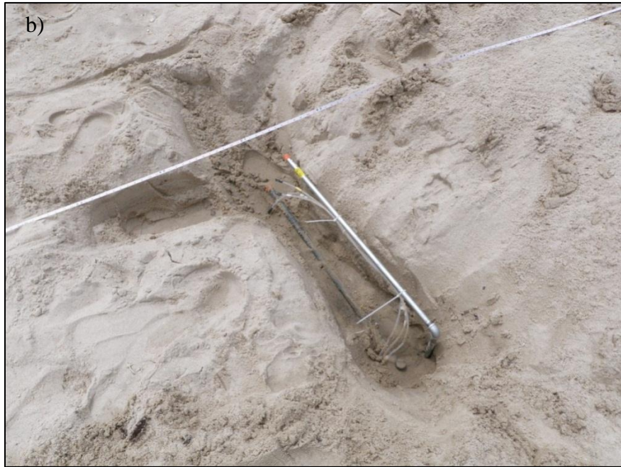
Figure A3. Image of a) sampling port and b) multi-level sampler after installation with tubing attached to steel pipe for retrieval.
