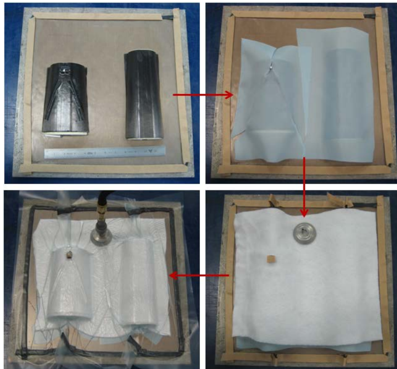
Figure 21: Vacuum bag process and materials
