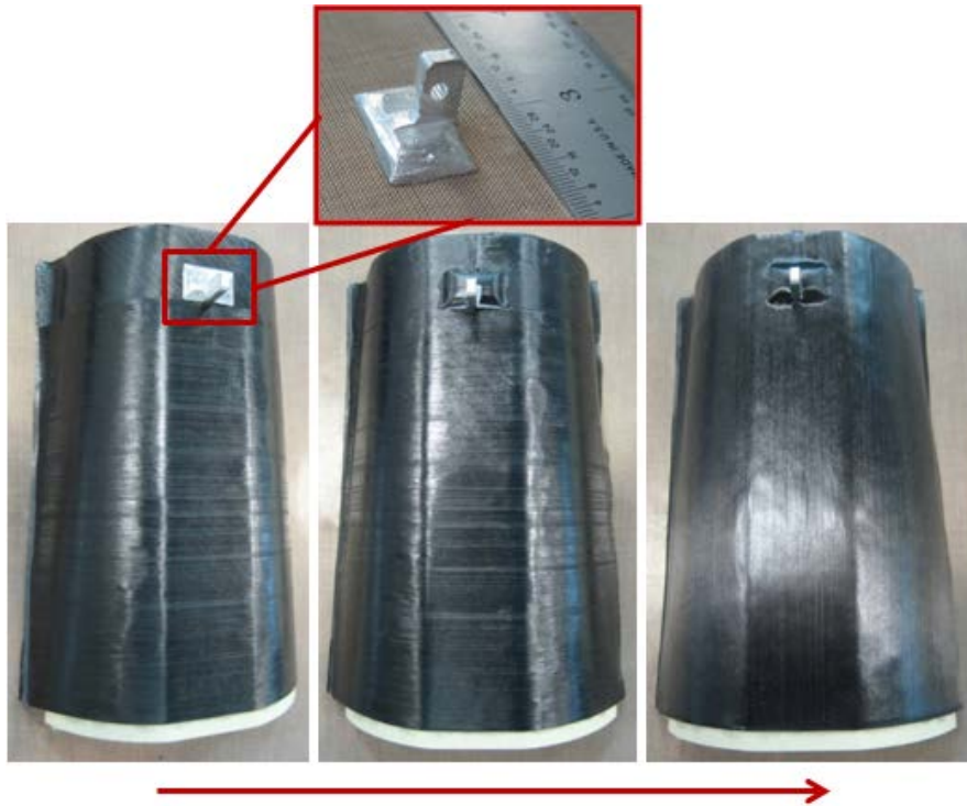
Figure 19: Layup process and cable termination block for upper arm mold
