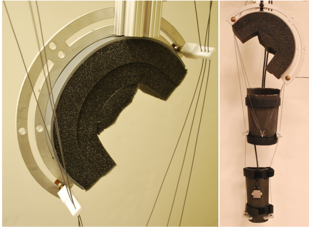
Figure 24: The shoulder cuff and full exoskeleton
