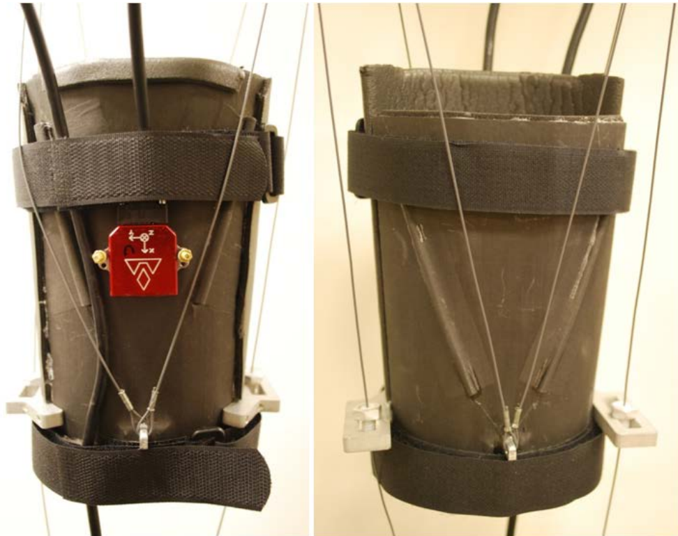
Figure 22: Outer (left) and inner (right) upper arm braces
