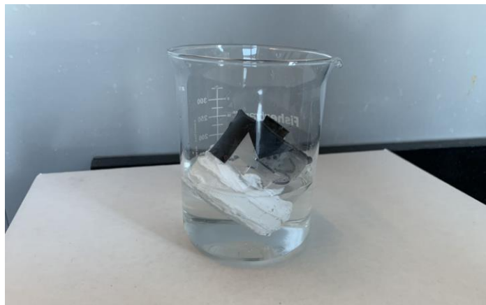
Figure 2.1 Experimental setup for Nafion115 on a counter-top at room temperature
