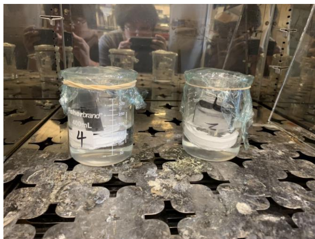
Figure 2.2 Experimental setup for Nafion115 in an oven at 40°C
