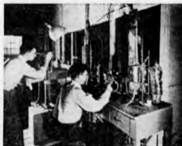
MEASURING pore-size distribution of porous media used in filtration: Harold P. Grace , B.S.Ch.E., Univ. of Pennsylvania '41; and Nym K. Seward , B.S.Ch.E., Lehigh U. '47.
