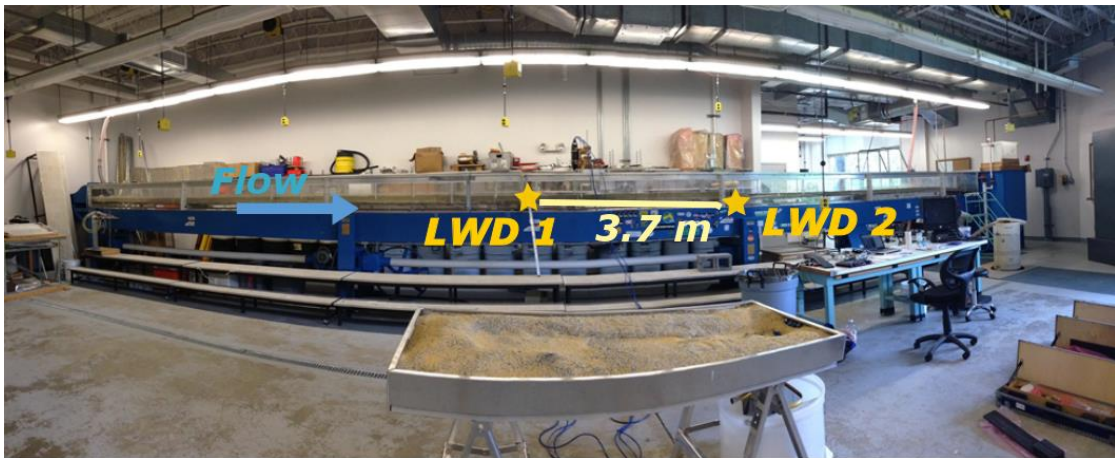
Figure 2.2 Photograph of the hydraulic flume used for the experiments. Flow directions and LWD locations are marked on the photograph.
