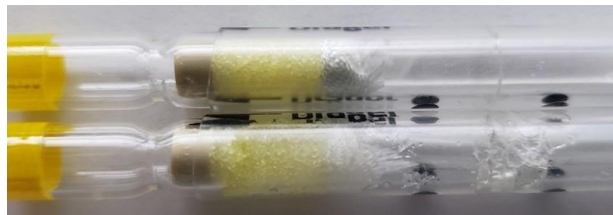
Figure 6: An unprocessed CST (top) and processed CST with slight discoloration in sponge (bottom).
