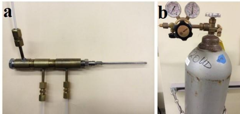
Figure 2.1 Photograph of 1 st generation coaxial setup. a: 1 st coaxial electrospinning nozzle; b: solution flow control device
