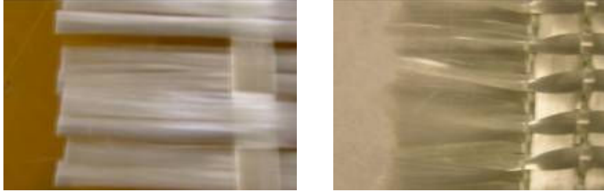
Figure 2.25: Woven and stitched E-glass, with 24 and 96 oz/yd 2 area weights respectively, highlight how much more difficult the latter is to mesh with multiple layers than the former.
