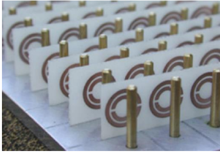
Figure 1.1: Split ring resonator fed by copper wire
