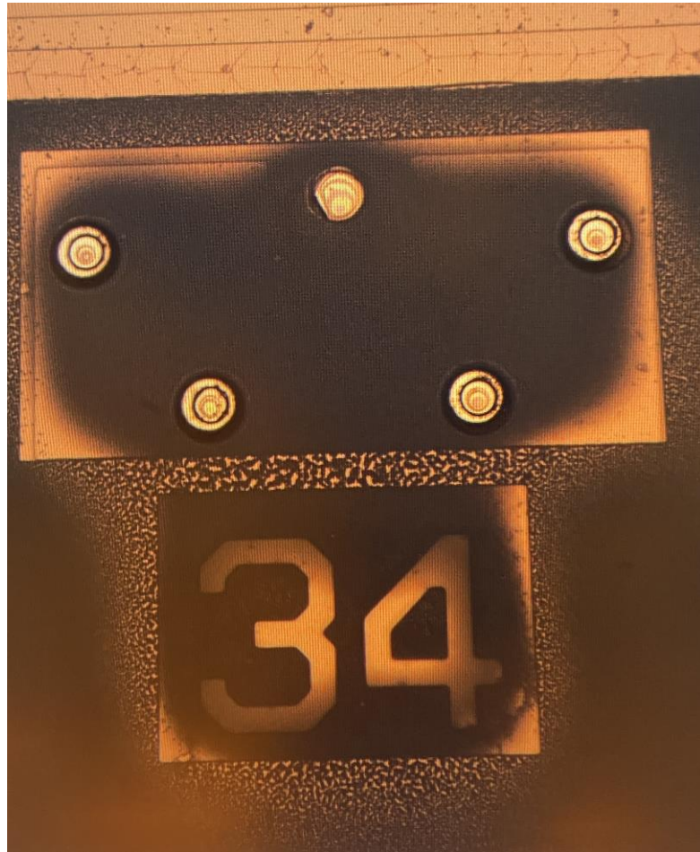
Figure 2.9. Seed layer for electroplating consisting of Ti, Au, and Ti.
