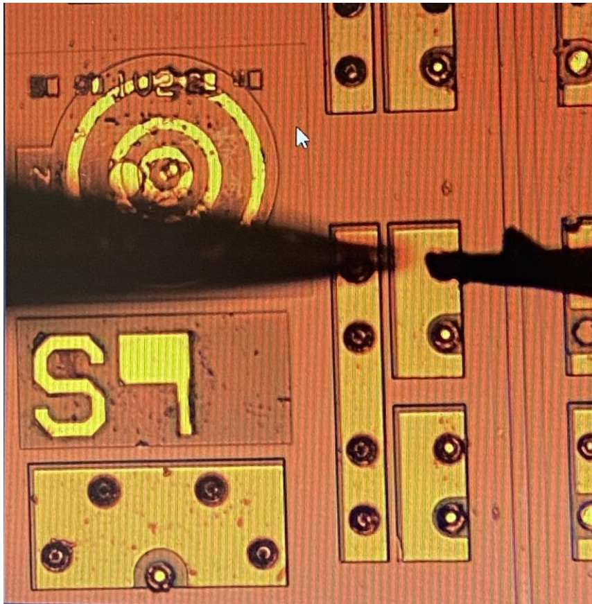
Figure 2.11. Completed flipped absorber devices undergoing IV curve testing after electroplating to verify normal functionality.
