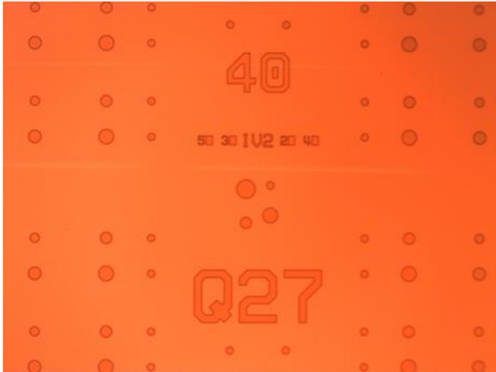
Figure 2.1. Lithography features for N-mesas are added on top of N-contact metal and SiO 2 hard mask.
